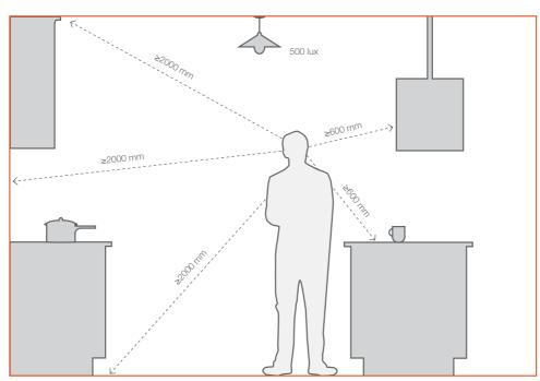
Normal viewing positions vary depending on the type of surface being inspected.
