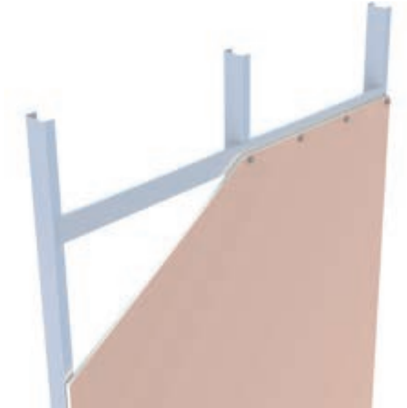
Nog on edge from ex 64mm x 30mm BMT track. Stagger nogs by at least 400mm on opposite sides of the wall.
